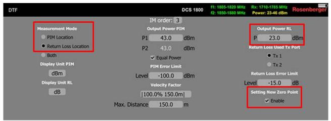
After successful zeroing "PASS" is displayed and with that the zero-point is set. To avoid mistakes in the following measurements please uncheck the "Enable" checkbox in the DTF settings screen. With that the "Zero RL" button on the measurement screen disappears.
