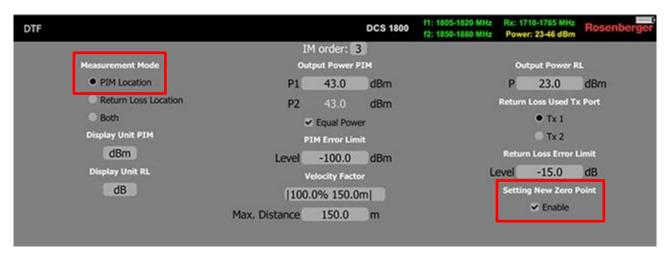
After that, connect the DTF Zeroing adaptor and a Low PIM load at the desired zero-point. To start zeroing PIM click on "Zero PIM" on the bottom of the DTF measurement screen.
