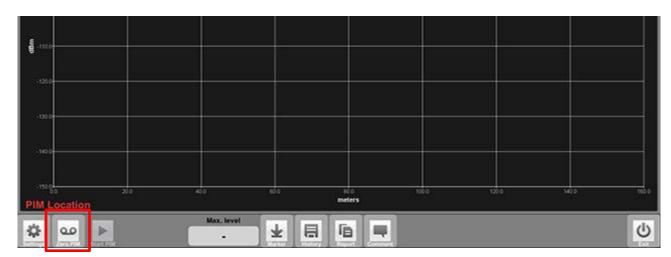
After successful zeroing "PASS" is displayed and with that the zero-point is set. To avoid mistakes in the following measurements please uncheck the "Enable" checkbox in the DTF settings screen. With that the "Zero PIM" button on the measurement screen disappears. The zeroing can also be used to set an offset.
