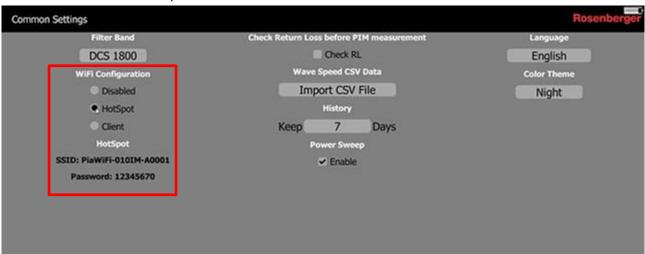
Open the WiFi connections screen on your tablet and connect with the network entitiled with the SSID shown on the PIM Site Analyzer  $\alpha$ . You will be prompted to input the network's password which also shown on your device's screen.
