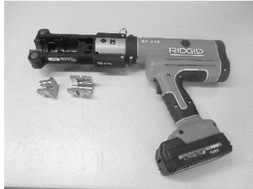
Cold Weld toolset: Rosenberger 11W119-C09/90 inserts with RIDGID tool RP 210/240 and Press Frameset 7/8"
